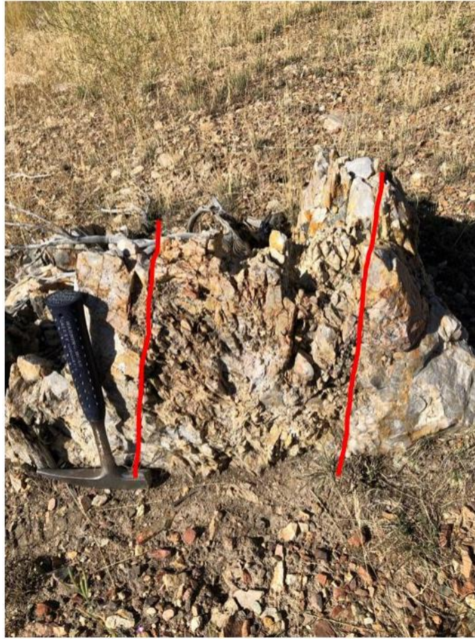
Figure 23: Tectonic Breccia Developed in Upper-Plate Vinini Formation; Evidence for Compressional Tectonics
